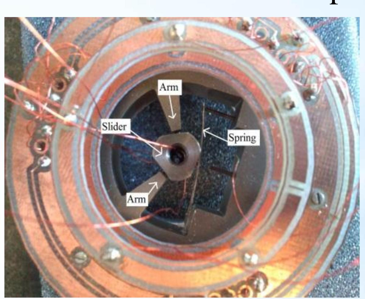
The slider will be used to approach the scanning tip to the specimen using stick-slip method.
