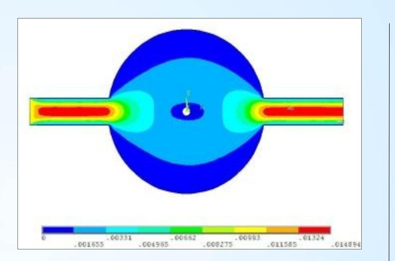
CFD analysis of the velocity gradient in the electrolytic cell in its top view. The sulfuric acid flows from left to right. The center dot represents the scanning tip.
