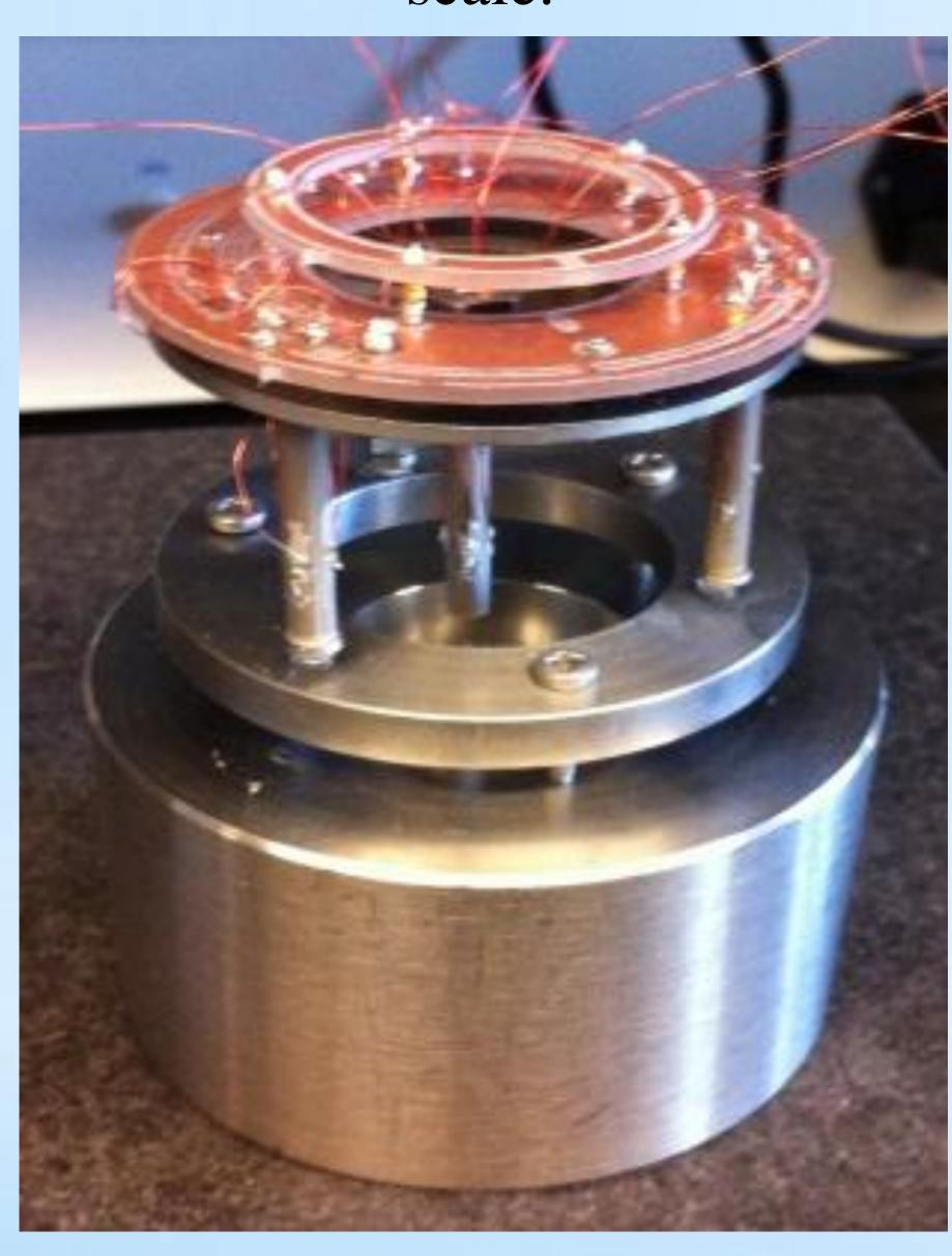
This AFM operates in a non-contact mode. The scanning probe is immersed in an electrolyte covering the specimen's surface. A topographic image is produced using a DAQ system (GXSM).
