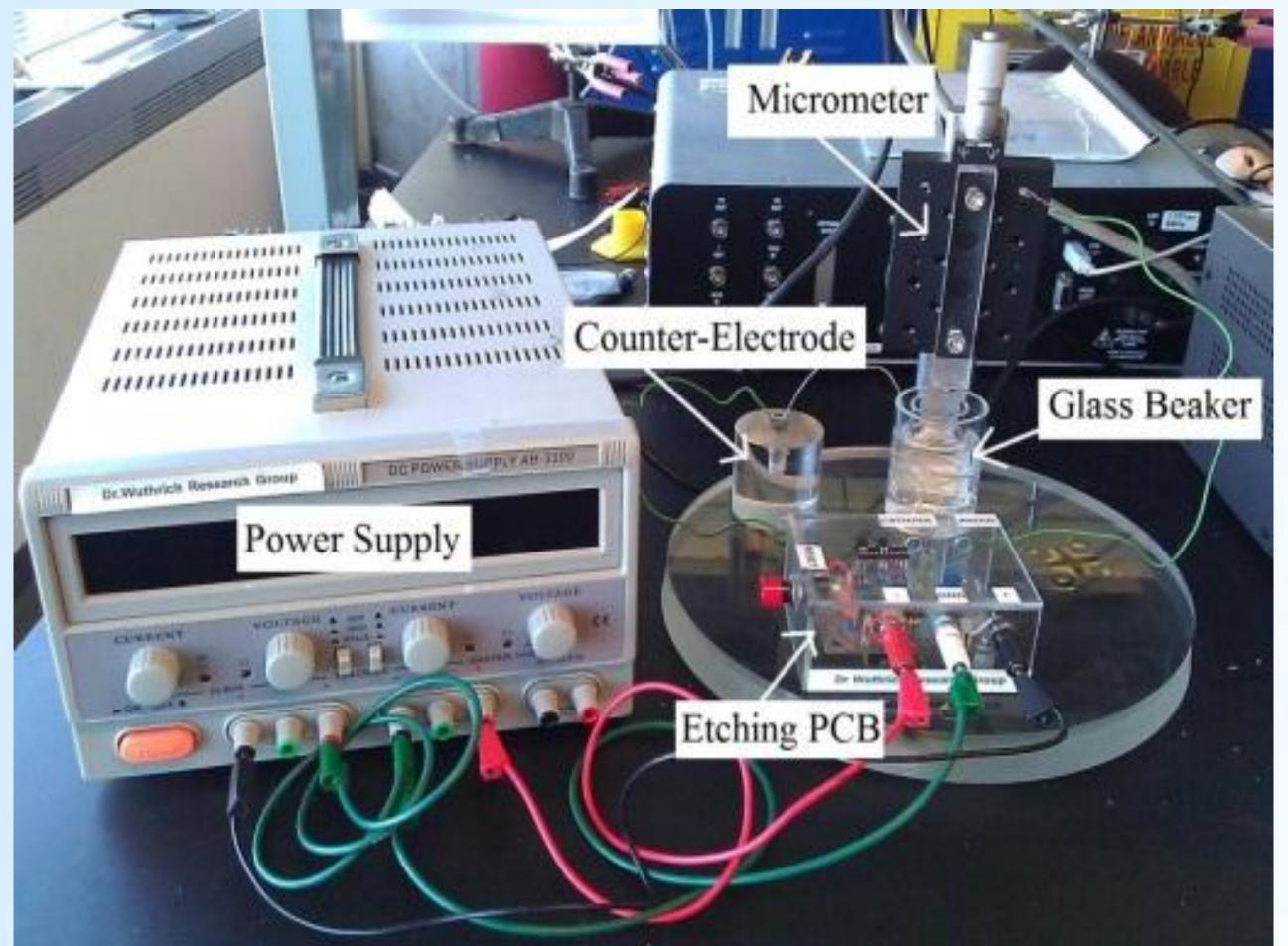
A tungsten wire is immersed in a KOH solution.
