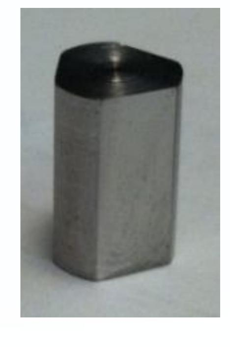
A high surface finished slider enhances the incremental steps induced by the stick-slip motion.
